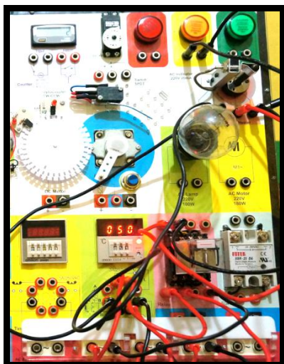
Figure 6. Temperature Control, Thermocouple, Relay, and Heater Testing
