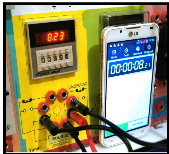
Figure 5. Timer on Delay Testing Source: personal document
